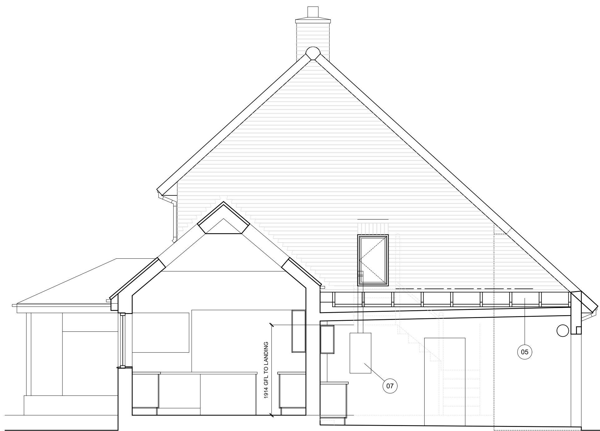
SECTIONAL SOUTH ELEVATION AA 1:50
